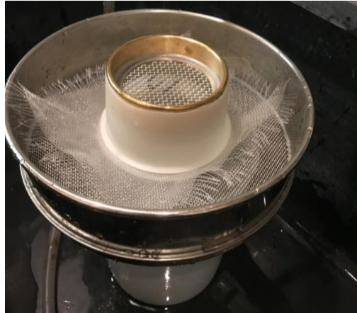
Figure 6: Wet sieving set up. A 2 mm sieve on top of a 1 mm sieve.
